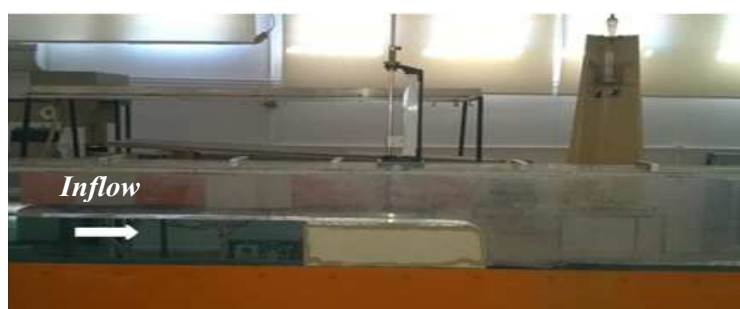
Figure 2: Laboratory equipment of the broad-crested weir and free-surface flow presentation.
