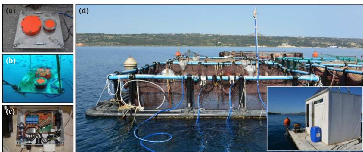
Figure 1. (a)–(b) Stainless steel plate for mounting the 38 and 120 kHz split-beam transducers below the fish cage (upwards-looking). (c) Raspberry Pi controller for the remote management of the acoustic system. (d) Operational installation of echosounders at the production cage; the inset image shows the anchored floating platform that hosted the EK80 transceivers and the peripheral electronic equipment.
